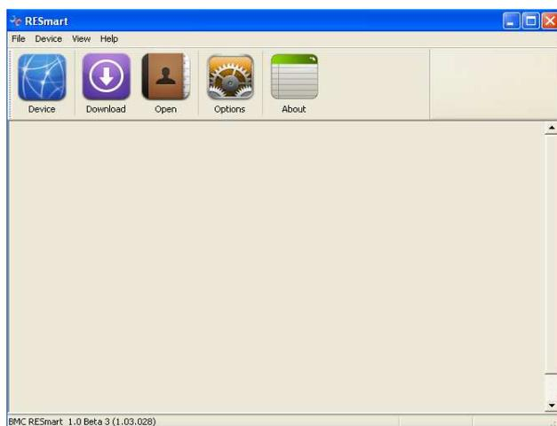
There is a menu bar on top of the screen where a tool palette with five frequently used buttons lies. The sub-window in the centre of the screen serves to display the data trend diagrams and statistical information of records. The status bar at the very bottom of the screen indicates present state of the software.
